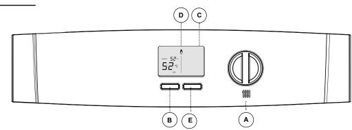
If an L code is shown on the display then the boiler can be restarted by pressing the Restart button (E).
